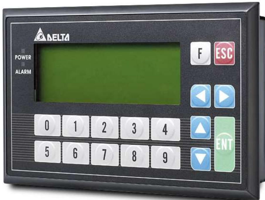
Figura N° 39: PLC Delta TP04P-32TP1R [20]
